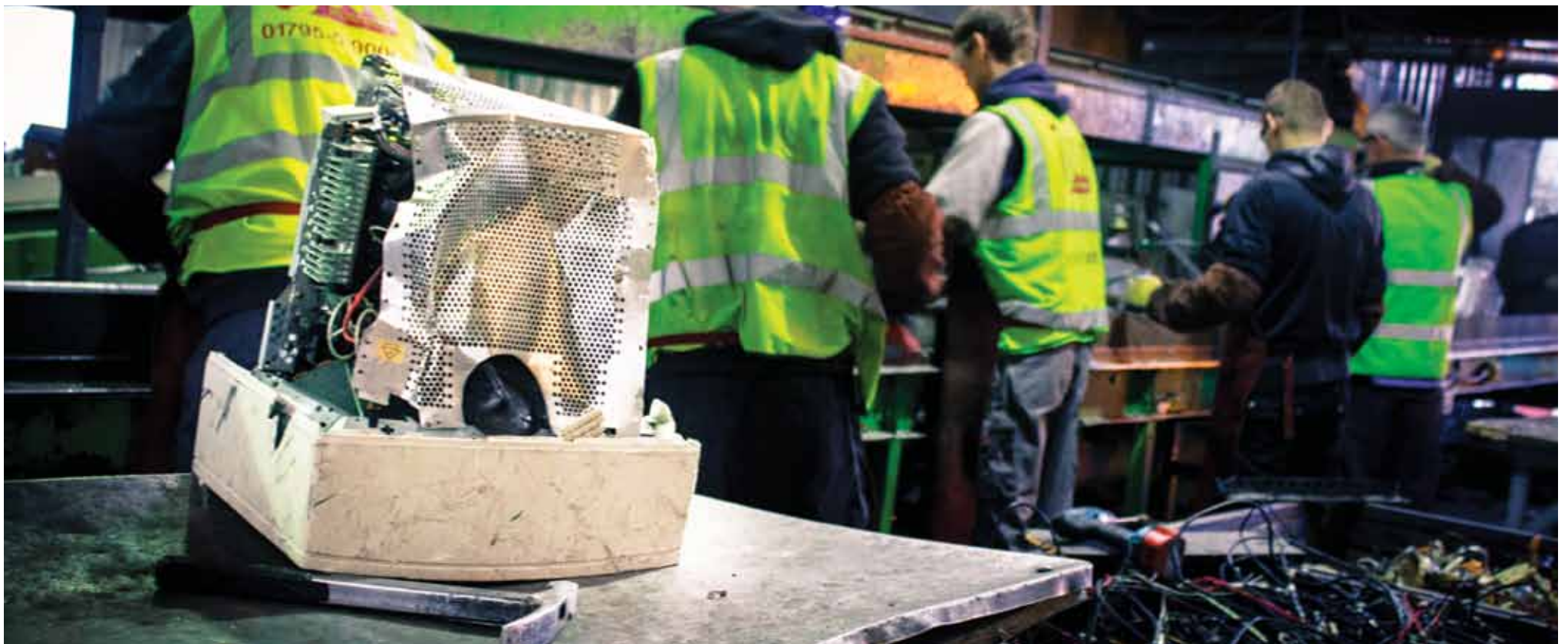
At Sweep in Kent computers and TVs with LCD screens must be taken apart by hand using brute force.
